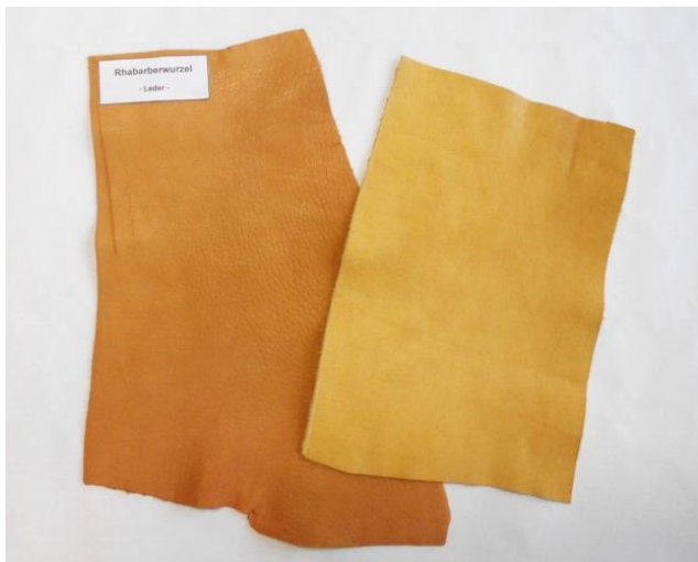
Picture 1: Pieces of wet-white re-tanned with Rhubarb and Polygonumextract
